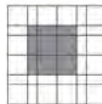
(E) 3 Piece 7x7 - 3% 7x14 - 32% 14x14 - 64% Laying Ratio: 1:4:4
